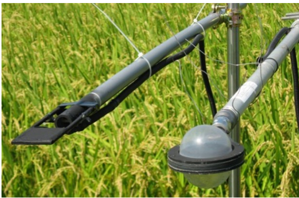
Photo 1 Net radiometers: TEC (left) and Q*7.1 (right) on top of the rice plants' canopy.
