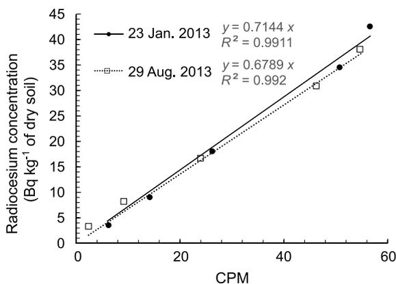
**Fig. 6** Temporal change in relationship between CPM by the proposed apparatus (Set A) and total radiocesium concentration. The samples were taken from a profile of a contaminated paddy field. The concentrations were corrected to the day when the CPM measurement was performed.
