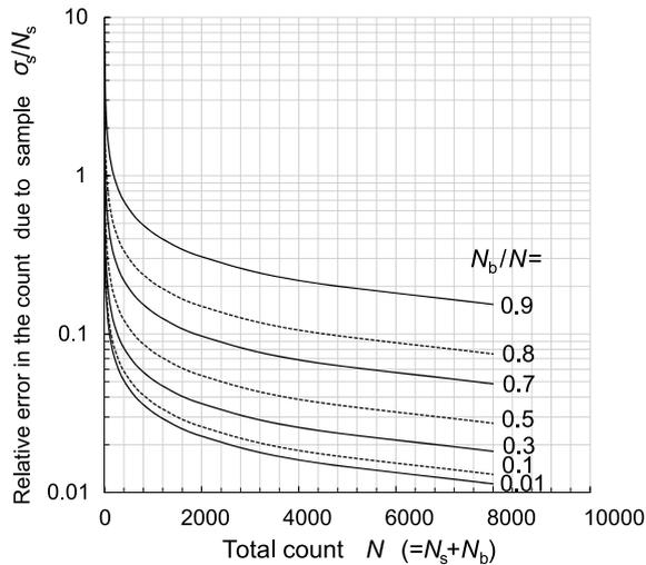
**Fig. 3** Theoretical estimate of relative error in the count due to sample  $N_s$  as a function of the proportion of the background radiation  $N_b$  to the total count  $N$ .
