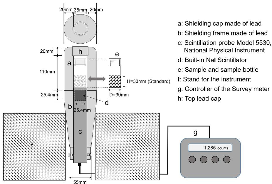
Fig. 1 Schematic of the proposed apparatus.
