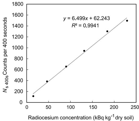
**Fig. 4** Relationship between total radiocesium concentration measured by Ge semiconductor detector and counts per 400 seconds by the proposed apparatus (Set A). The sample was the mixture of sediment in an agricultural reservoir and non-contaminated upland soil. The temporal decay of the concentration is corrected based on the date of the measurements.
