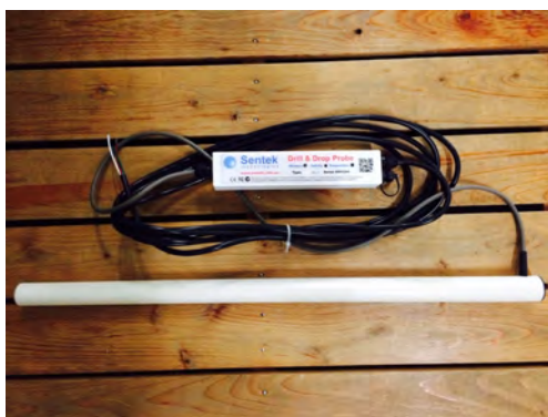
Fig. 2 60cm 長の Drill & Drop Probe. 60 cm length Drill & Drop Probe.
