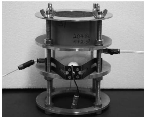
Fig. 6 Photo of tools set-up for  $k_a$  measurement.
