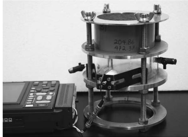
Fig. 2 Photo of the diffusionmeter apparatus.
