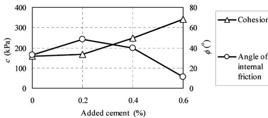
**Fig. 12** Variation of *c* and  $\phi$  of soil-cement with different cement content.
