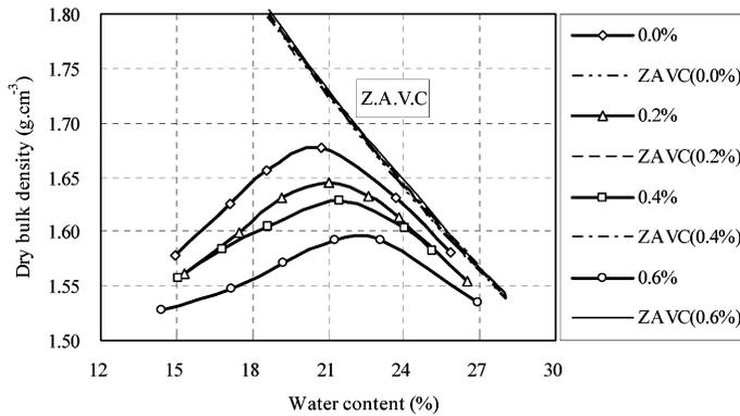
Fig. 5 Compaction curves of soil-cement with different cement content. (Z.A.V.C. means zero air void curve)
