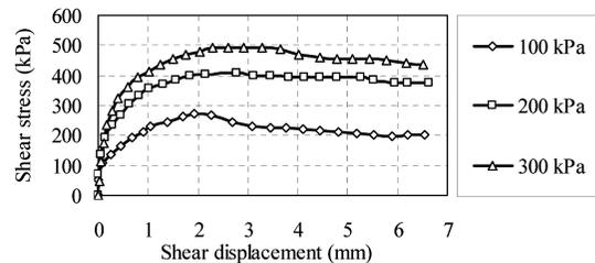
Fig. 8 Shear stress vs. shear displacement (0.2% soil-cement).
