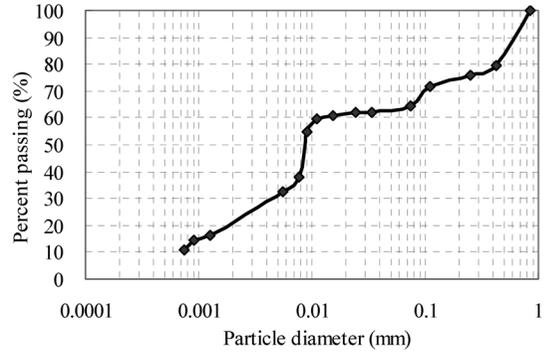
Fig. 1 Particle size distribution curve of soil.
