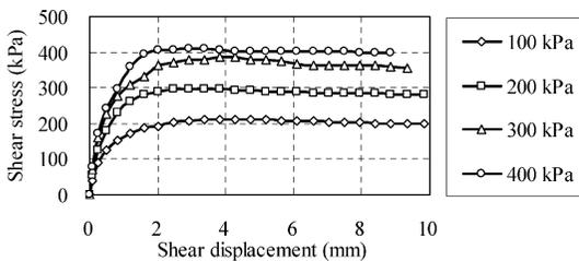
Fig. 7 Shear stress vs. shear displacement (0% soil-cement).
