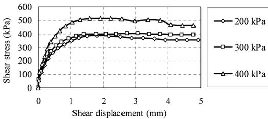
Fig. 9 Shear stress vs. shear displacement (0.4% soil-cement).
