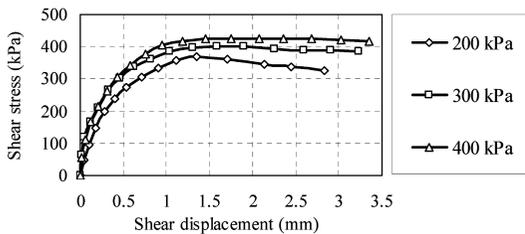
Fig. 10 Shear stress vs. shear displacement (0.6% soil-cement).
