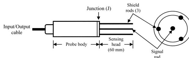
Fig. 1 A schematic diagram of the ADR probe.
