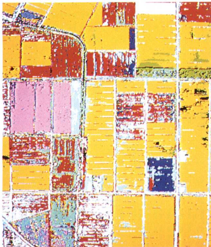
Photo. 2 Land-cover classification in dry fields area converted from paddy fields. (by digital image data from aerial infrared-color film)
